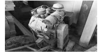
1983 CRAFCO ROUTER, MODEL W2-1230 SN 6064199, Machine is not being used no safety switches.
